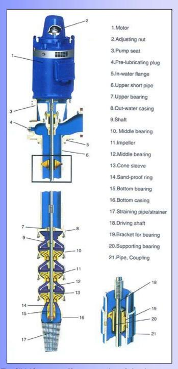
The SILI JC seawater lift pump consists of electric motor, coupling, line shaft, and impeller, bearing impeller cone for each stage impeller assembly and so on.
