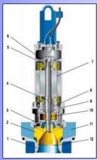
converted pressure energy. The rotational movement diverts the fluid flow in axial direction. The casing wear ring (12) prevents fluid any from flowing back from the casing into the inlet of the pump casing. At the rear side of the impeller, the shaft enters the casing via the discharge cover (3). The shaft passage through the discharge
